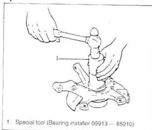
FIG. 4D — 16 PRESS-FITTING BEARING
